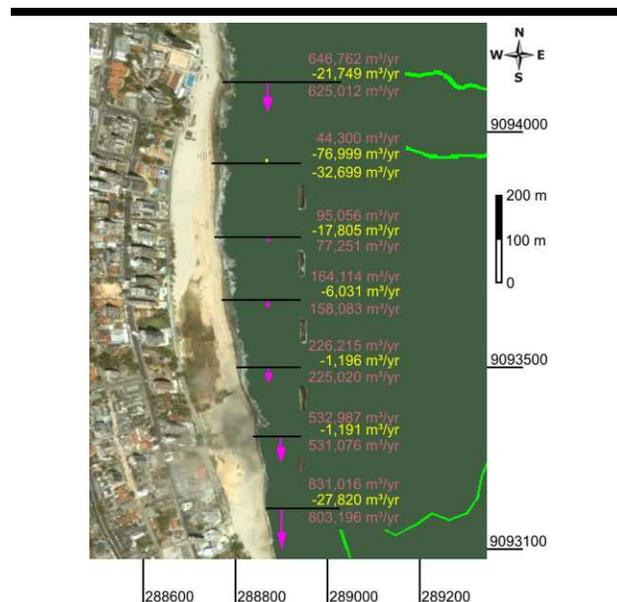
Figure 14: Calculated annual mean sediment transports in selected beach profiles along the studied area for the present breakwater configuration. By convention, the south bound transport is defined as positive, which are represented with a magenta arrow; the negative transports to the north are represented in yellow. The numbers to the right show the annual transport for each direction, with the mean transport shown below of each beach profile line.
