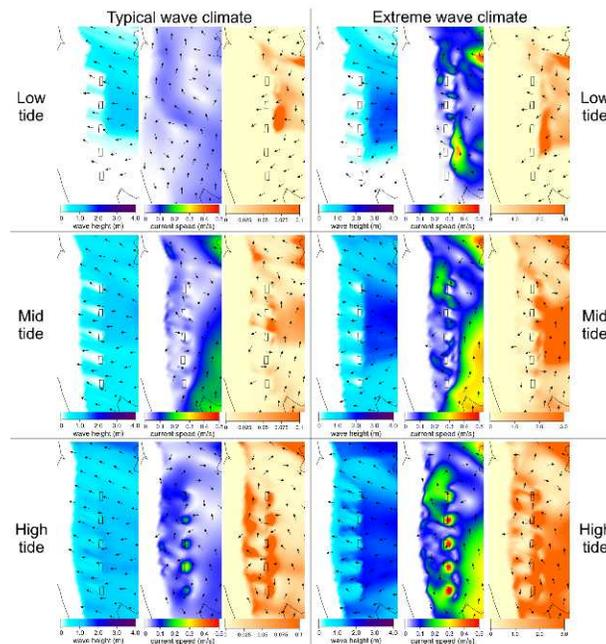
Figure 11: Simulation results for the present breakwater configuration, in both typical (left side) and extreme (right side) wave climate conditions (table 1). From top to bottom the lines show the low tide, mid tide and the high tide results. For each half line side it is displayed the wave height, current speed and sediment transport results for each wave climate condition.
