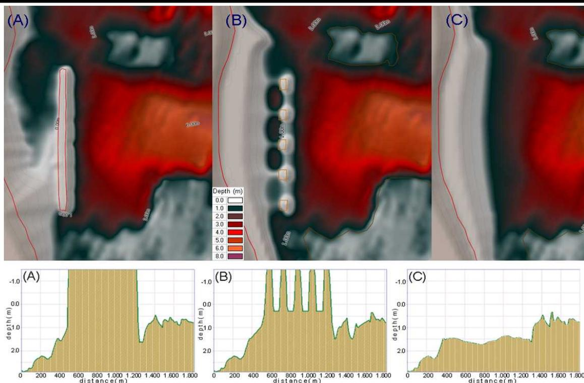
Figure 9. Three different configurations and a scenario of the study area (A) former breakwater configuration, (B) present breakwater configuration and (C) without breakwater scenario.
