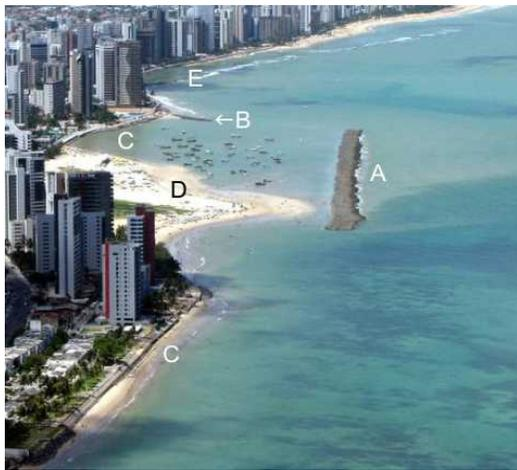
Figure 4. Jabotão dos Guararapes coastline, showing the high density occupation of the study area (A) the detached breakwater, installed in the region in its first configuration, (B) the small groin, (C) the already sand depleted areas with seawall protections, (D) the trapped sand salience and (E) the eroded area to the north. (photo: Roberto Angelo).
