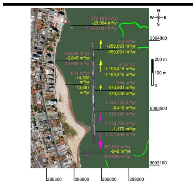
Figure 13. Calculated annual mean sediment transports in selected beach profiles along the studied area for the former breakwater configuration. By convention, the south bound transport is defined as positive, which are represented with a magenta arrow. The negative transports to the north are represented in yellow. The numbers to the right show the annual transport for each direction, with the mean transport shown below of each beach profile line.
