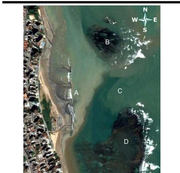
Figure 2. Candeias Beach showing the studied breakwater (A) still being modified to its present configuration, (B) the patch reef known as abreus, (C) the Abreus bar and (D) the fringing reef formation which protects most part of the beach (source: Google Earth, July, 2013).
