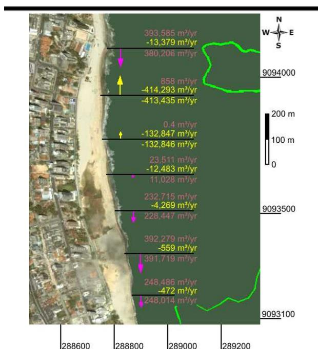
Figure 15. Calculated annual mean sediment transports in selected beach profiles along the studied area for the scenario without breakwater. By convention, the south bound transport is defined as positive, which are represented with a magenta arrow; the negative transports to the north are represented in yellow. The numbers to the right show the annual transport for each direction, with the mean transport shown below of each beach profile line.
