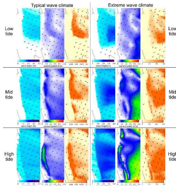
Figure 12: Simulation results for the scenario without a protective breakwater, in both typical (left side) and extreme (right side) wave climate conditions (table 1). From top to bottom the lines show the low tide, mid tide and the high tide results. For each half line side it is displayed the wave height, current speed and sediment transport results for each wave climate condition.
