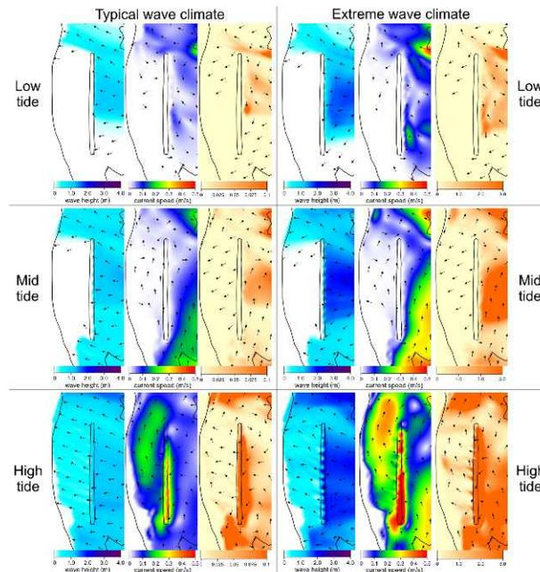
Figure 10: Simulation results for the former breakwater configuration, in both typical (left side) and extreme (right side) wave climate conditions (table 1). From top to bottom the lines show the low tide, mid tide and the high tide results. For each half line side it is displayed the wave height, current speed and sediment transport results for each wave climate condition.
