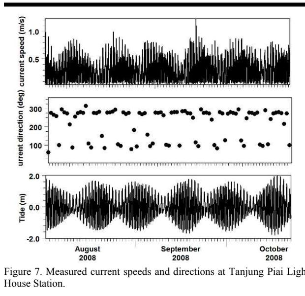
Figure 7. Measured current speeds and directions at Tanjung Piai Light House Station.
