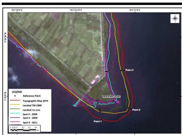
Figure 2. Shoreline changes due to coastal erosion at Tanjung Piai from 1974 to 2011 (DID, 2013).
