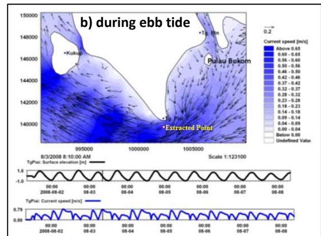
Figure 15. Current speeds around Tanjung Piai: a) during flood tide (0.1 - 0.3 m/s); b) during ebb tide (0.3 - 0.6 m/s) (Wan Hasliza *et al.*, 2013).
