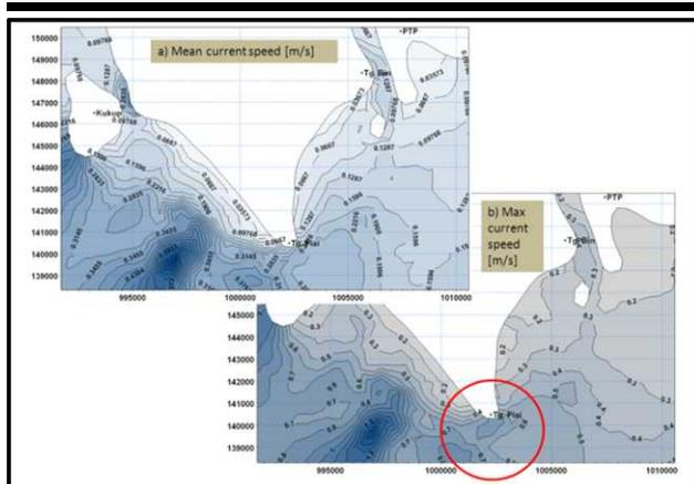
Figure 14. Statistical analysis of current speed forced by tide and wind: a) mean current speed; b) maximum current speed in the study area; red circle indicates that Tanjung Piai is subjected to a maximum current speed of more than 0.6 m/s (Wan Hasliza *et al.*, 2013).
