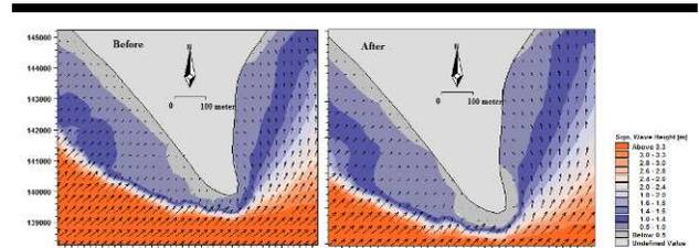
Figure 19. Difference in the modelled significant wave height, before and after the implementation of the proposed structure.
