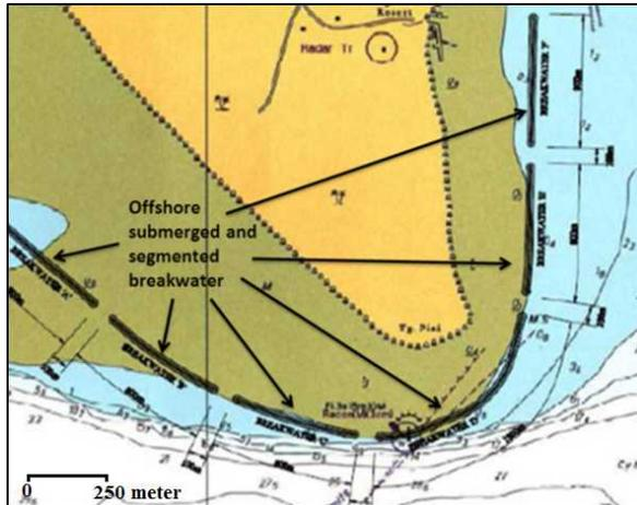
Figure 9. Proposed offshore, submerged and segmented breakwaters to minimise erosion (DID Malaysia).
