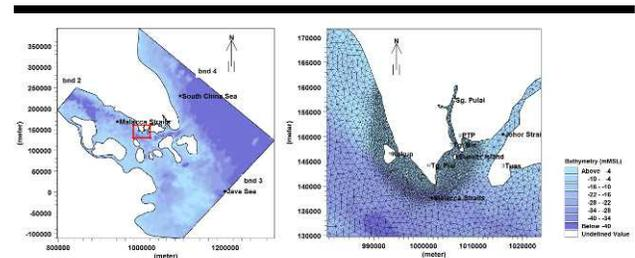
Figure 8. Boundary condition and computational mesh.
