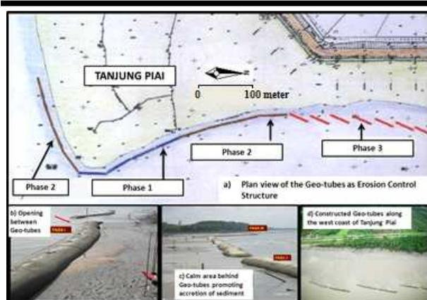
Figure 10. Geo-tubes along the Tanjung Piai coast: (a) plan; (b) opening between geo-tubes; (c) calm area behind the geo-tubes promoting accretion of sediment; (d) geo-tubes along the east coast of Tanjung Piai, seen from above (DID Malaysia).
