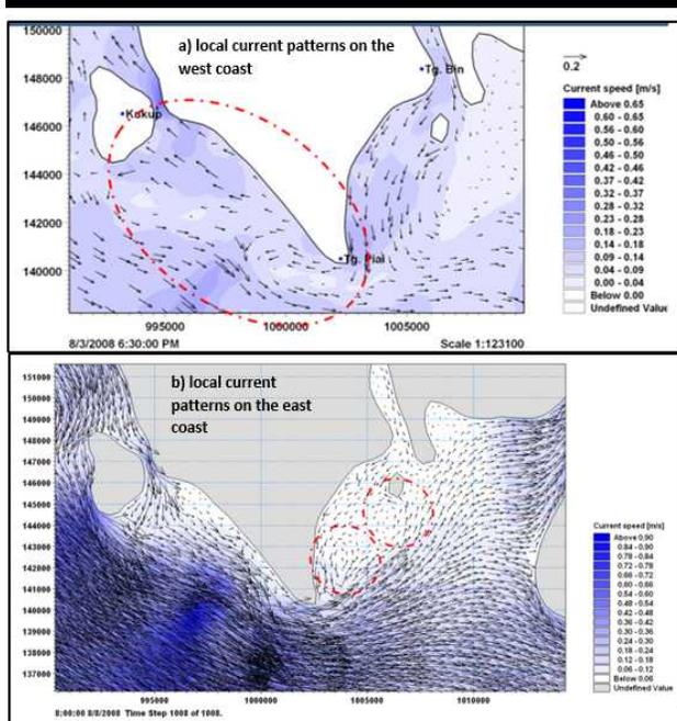
Figure 16. Local current patterns (red circles) at the: a) west coast; b) east coast of Tanjung Piai, formed by the existing islands located around Tanjung Piai (Wan Hasliza *et al.*, 2013).
