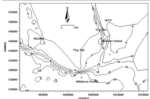
Figure 4. Measured bathymetry in meters referred to Mean Sea Level (MSL).
