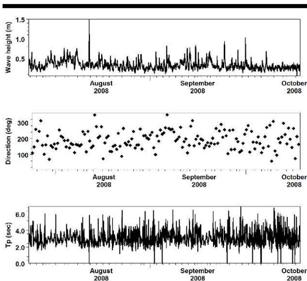
Figure 5. Measured wave height, direction and period at Tanjung Piai Light House Station.
