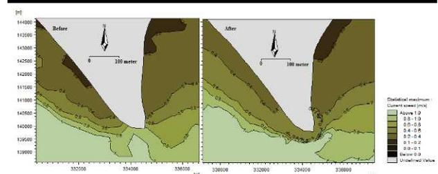
Figure 18. Difference in the modelled current speed, before and after the implementation of the proposed structure.
