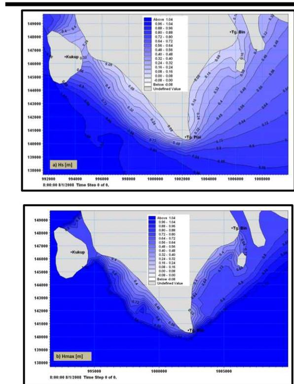
Figure 17. Statistical analysis of: (a) significant wave height; (b) maximum wave height in the study area (Wan Hasliza *et al.*, 2013).
