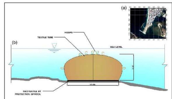
Figure 12. Location and cross-section of the submerged structures.
