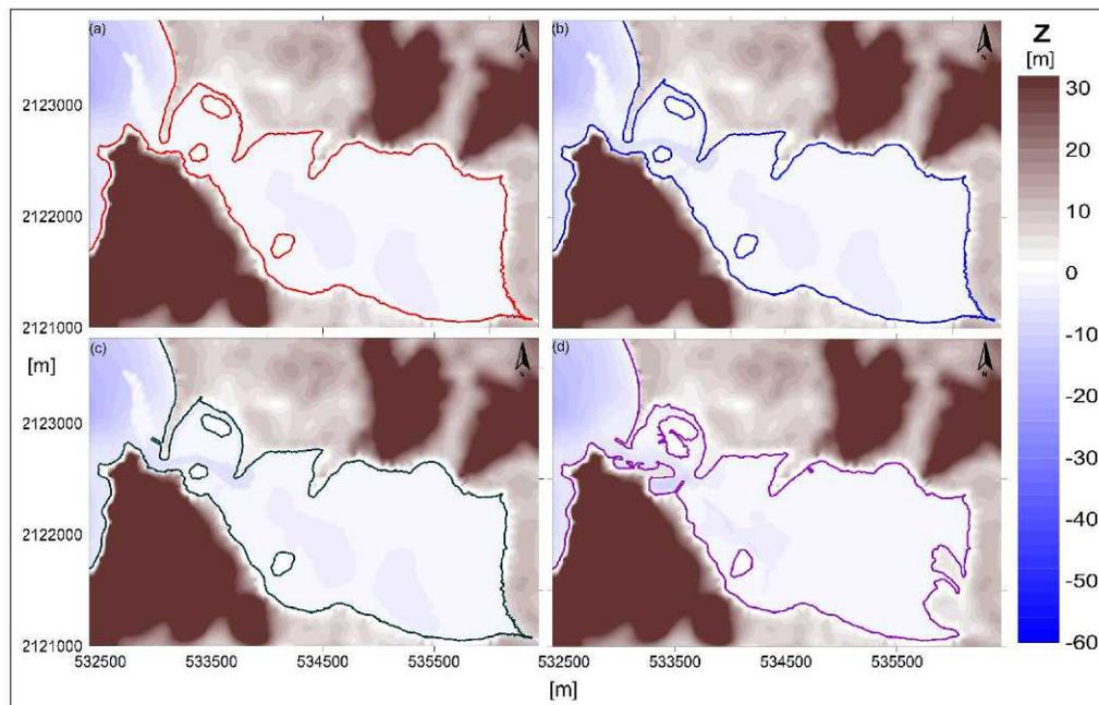
Figure 8. Constructed bathymetries for (a) 1983; (b) 1986: inlet dredged; (c) 1986: breakwater in situ and (d) 2013.
