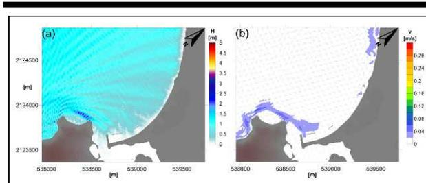
Figure 13. Hydrodynamics imposed by the proposed solution (a) wave field and (b) wave induced currents.
