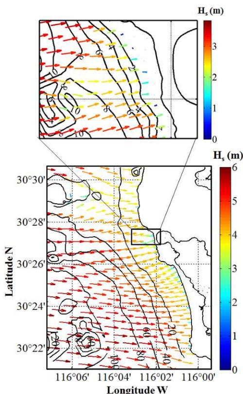
Figure 7. Wave propagation results from the Delft3D model for the most frequent storm waves of  $H_s$  of 5 m,  $T_p$  of 8 s and a wave direction of  $275^\circ$  at boundary condition. The top panel is a close up of the bottom panel for the barrier breaching location.
