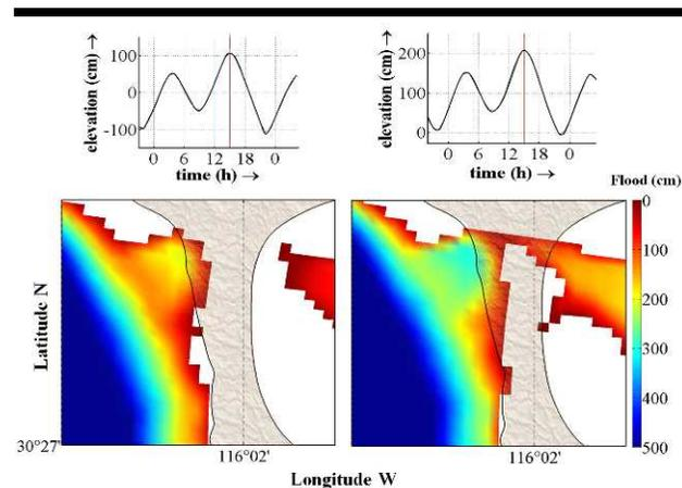
Figure 8. Barrier overtopping and overwashing during high spring tides and extreme wave conditions of  $H_s$  of 5 m,  $T_p$  of 8 s from  $275^\circ$  without storm surge (left panel) and for the same conditions and 1 m of storm surge (right panel). The modeled area corresponds to the rectangle in Figure 1.
