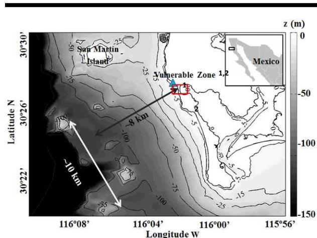
Figure 1. Location of San Quintin within Mexico (top right panel) and the offshore and nearshore bathymetry. The most vulnerable location for barrier breaching (red box) and the location of the meteorological station (blue triangle) are shown.
