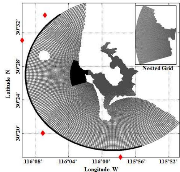
Figure 3. Large grid and nested grid used to propagate waves and flows. The coastal boundary is closed and the ocean boundary is opened with absorbance characteristics. The thicker line represents the opened offshore boundary forced with tides and wave conditions. Diamonds are linked to sites of observational wave data from the PACE grid.
