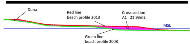
Figure 15. Comparison between beach profiles 2008 when dune was finished and 2013.
