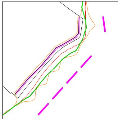
Figure 17. The hold “zero line” is represented in red, the thick green line shows the shoreline after six years and the wavy orange line represents expected salients.
