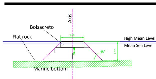
Figure 11. Breakwater cross section.
