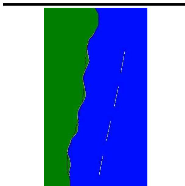
Figure 7. Beach response under normal wave conditions, the black line corresponds to the original coastal line and the green salient corresponds to the shape generated by the presence of breakwaters.
