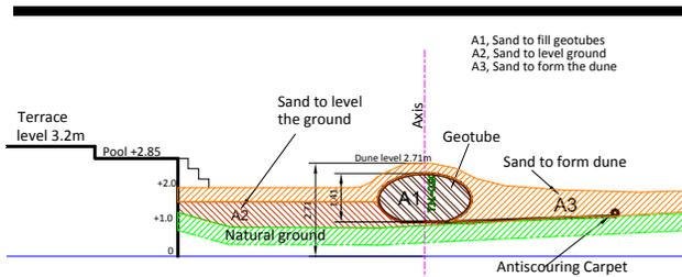
Figure 12. Cross section of constructed artificial dune.
