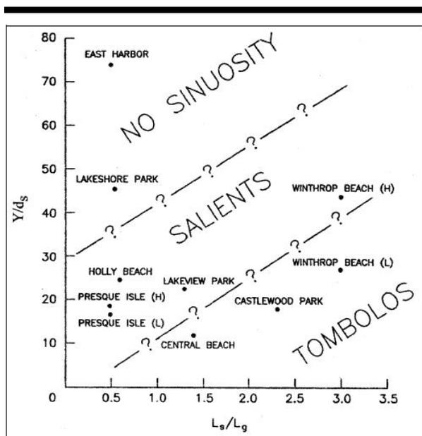
Figure 9. Conditions for formation of salients and tombolos (Coastal Engineering Manual, 2006),  $L_s$  represents the structure length,  $L_g$  the length of gap,  $Y$  is the distance from shore and  $d_s$  is the depth at which the structure is located.
