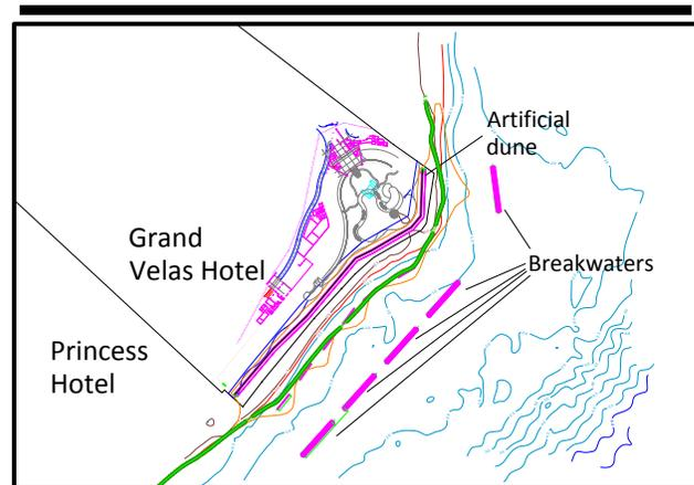
Figure 10. Coastal protection project with the five breakwaters and an artificial dune.
